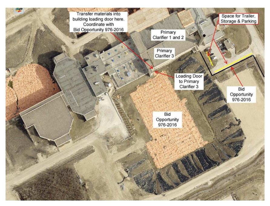
SEWPCC – PRIMARY CLARIFIER TRAVELLING BRIDGES REFURBISHMENT SITE PLAN
